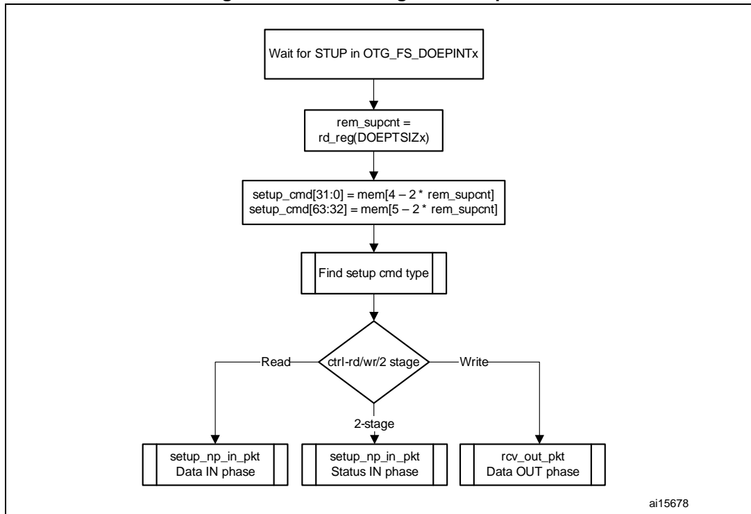
Figure 259. Processing a SETUP packet
