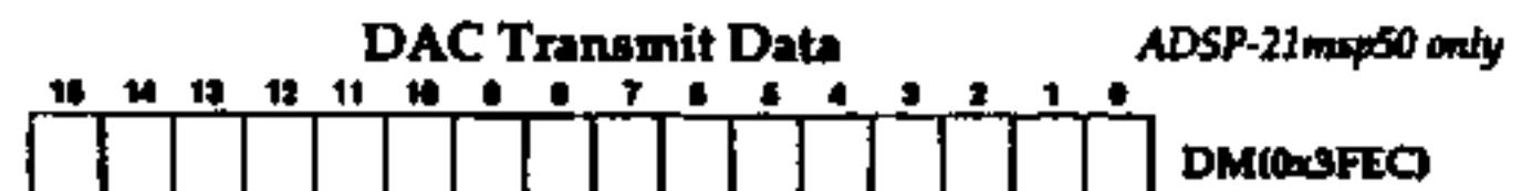
No registers are located between DM(0x3FEC) and DM(0x3FE8)
